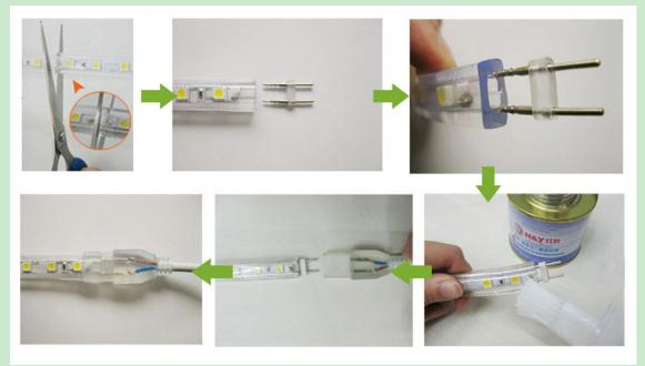
After cutting the the strips, First insert the small pin, After making it tightly, Then taken some PVC glue to the strips, Then insert the power plug tightly, It can be working now.
