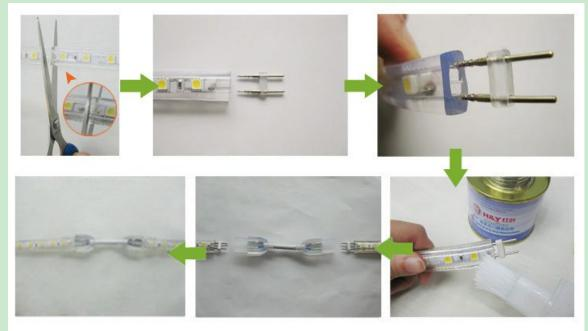
After cutting the strips, First insert the small pin, Once insert tightly, Then taken some PVC glue on the strips, At last ,Insert the middle connector, It is ok now.
